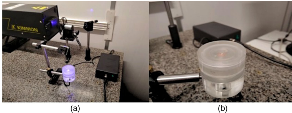
FIGURE 2 Apparatus used to determine the thermal diffusivity of kernel pericarp via open photoacoustic cell (OPC), (a) operating equipment and (b) photoacoustic chamber with an electret microphone
